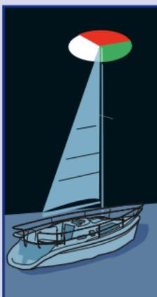
*An alternative to the sidelights and sternlight is a combination red, green and white light, which must be exhibited near the top of the mast.*
